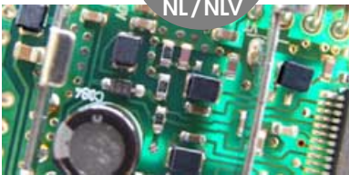
Application example of digital TV tuner and tuner IC signal lines
