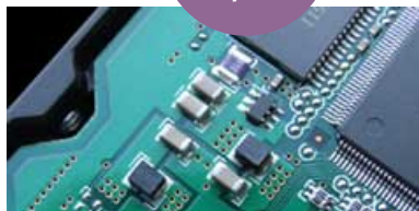
Application example of ATA-compatible HDD and HDD controller VDD line
